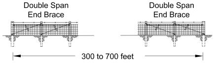
3. Use line braces to divide fence lengths where runs of fence are more than 700 feet long. a run is the distance between a corner, end or gate post and the next corner, end, or gate post.
