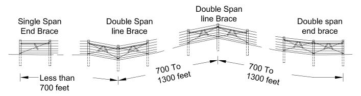
Drawing not to scale. Standardized drawing must be adapted to the specific site.
