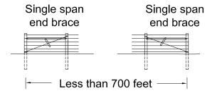
2. Use double span brace assemblies for runs of fence that are 700 to 1300 feet between corner, end, and/or gate posts.
