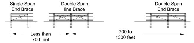
4. On uneven terrain, locate line braces at the top and bottom of each hill.
