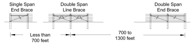
4. On uneven terrain, locate line braces at the bottom of each hill.
