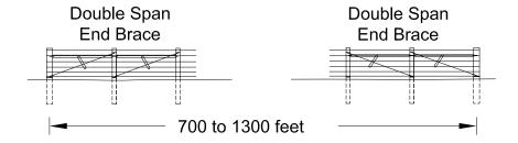
3. Use line braces to divide fence lengths where runs of fence are more than 1300 feet long. A run is the distance between a corner, end or gate post and the next corner, end, or gate post.
