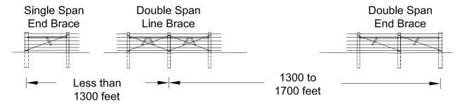
4. On uneven terrain, locate line braces at the bottom of each hill.
