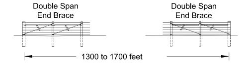
3. Use line braces to divide fence lengths where runs of fence are more than 1300 feet long. A run is the distance between a corner, end or gate post and the next corner, end, or gate post.
