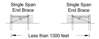
2. Use double span brace assemblies for runs of fence that are 1300 to 1700 feet between corner, end, and/or gate posts.
