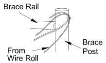
Drive staple about half its length into brace post about 4 inches above Brace Rail, on opposite side from brace.  Drive staple in a similar manner on Anchor Post about 4 inches above ground, on opposite side from Brace.  Unroll enough Brace Wire for two complete loops around Anchor and Brace Posts. Thread Brace Wire through staples.
