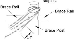
5. Cut Brace Wire from roll, allowing enough wire to wrap around Brace Post and extend 6 to 12 inches past the other wire end. Splice wires together.
