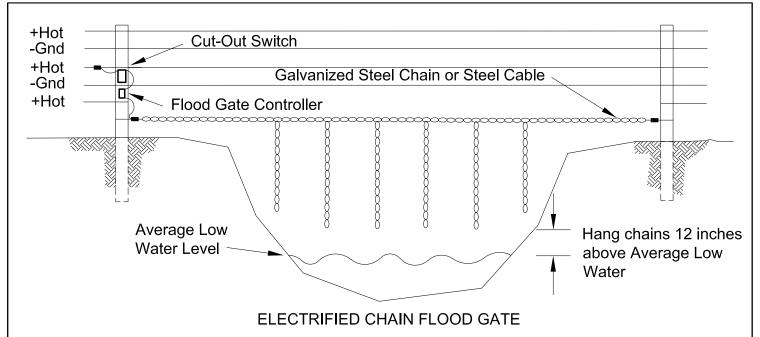
Stretch a galvanized chain or steel cable between two fence posts (one on each side of the stream). Attach lengths of galvanized chain so that they hang approximately 12 inches above the elevation of average low water. Space the vertical sections of chain at 6 inches apart for small livestock and up to 12 inches apart for larger animals.
